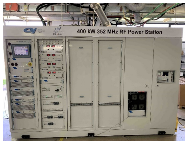
Figure 2: The complete amplifier.
