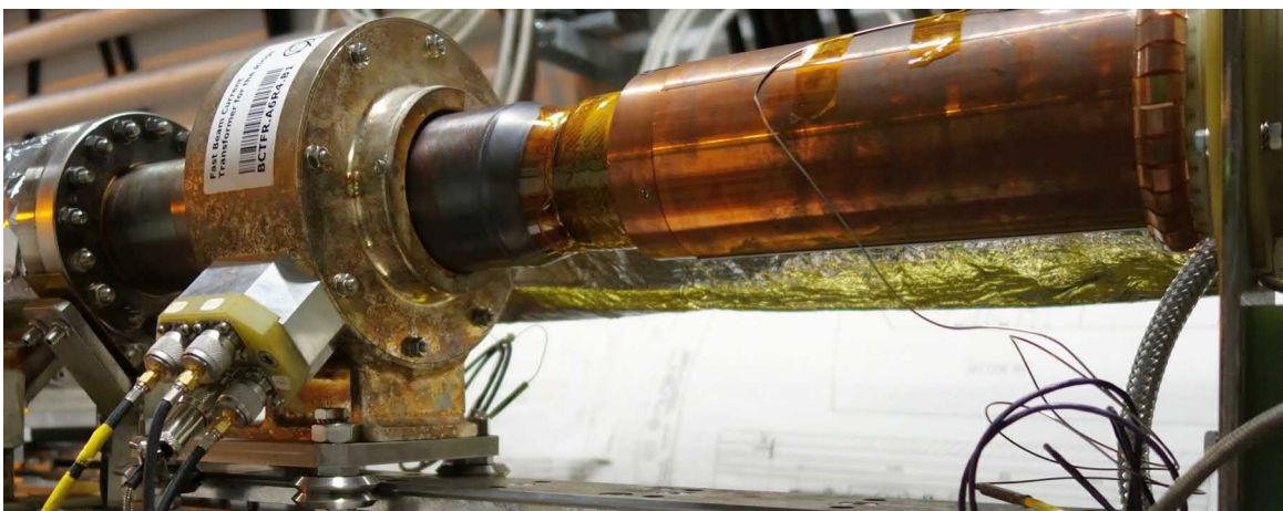
Figure 4.20: FBCT R1A installed in the measurement position.
