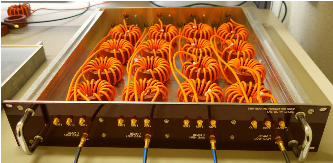
Figure 3.26: Sixteen electrically-insulated common-mode chokes installed in a common enclosure to serve two WCTs.
