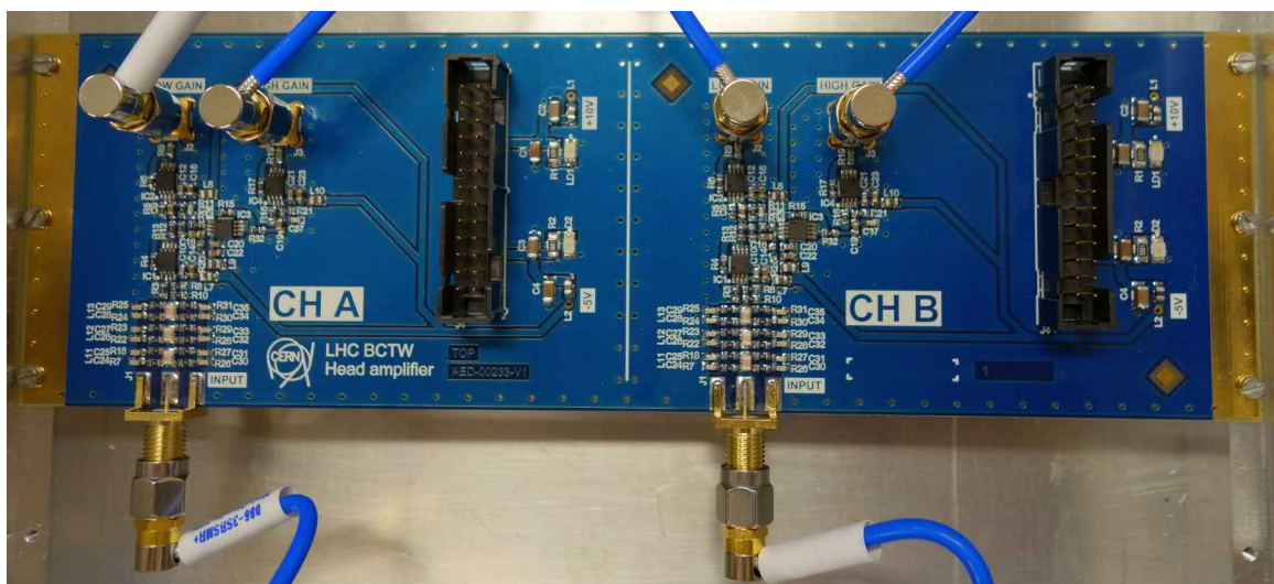
Figure 3.18: An assembled head amplifier PCB installed in an enclosure.
