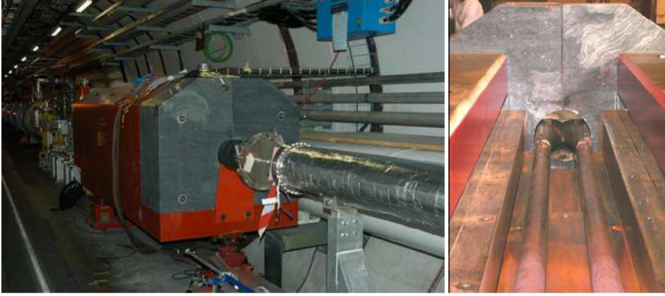
Figure 2.6: Pictures of the TAN absorber, positioned at about 141.5 meters from the interaction point IP1. On the left, it shows the TAN fully assembled in the LHC tunnel as viewed from the direction of the IP1. On the right, there is a depiction of the TAN during its assembly at CERN, viewed from above facing the IP. A 96mm gap between the two beam pipes is included to accommodate the installation of the LHCf detectors.
