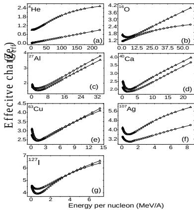
**Fig 1:** A plot of effective charge state of projectile such as  $^4\text{He}$ ,  $^{16}\text{O}$ ,  $^{27}\text{Al}$ ,  $^{40}\text{Ca}$ ,  $^{63}\text{Cu}$ ,  $^{107}\text{Ag}$  and  $^{127}\text{I}$  on targets such as  $^{208}\text{Pb}$  and  $^{238}\text{U}$  with ion energy per nucleon.
