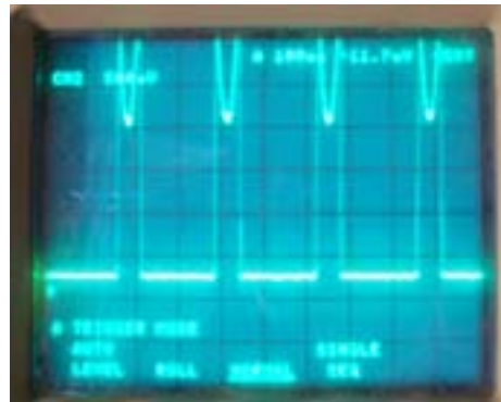
Figure 3: A photogate signal as read out on an oscilloscope
