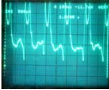
Figure 10: Baseline fluctuation on the oscilloscope readout
