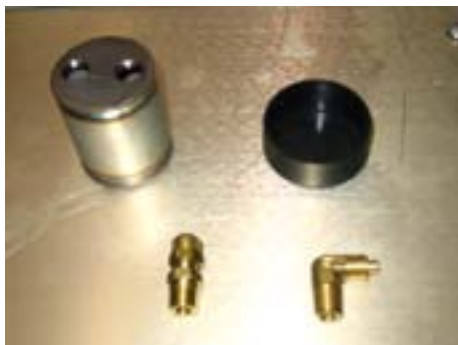
Figure 5: Oil trap components clockwise from top-left: Metal Oil Trap, Endcap, Elbow Connector, Straight Connector
