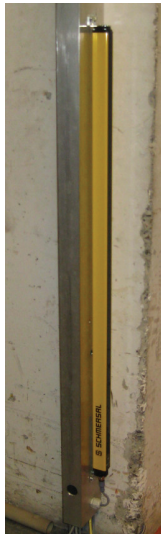
(a) The emitter of the light grid system.
