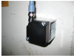
(d) The combined emitter and acceptor element of the light barrier.
