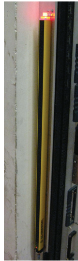
(c) The red light of the acceptor shows that someone has interrupted the signal.
