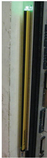
(b) The acceptor of the light grid has a green light to show that nobody was detected by the system.
