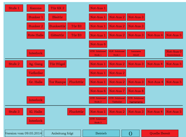
Figure 5: This screen shows the three levels of the personnel interlock subsystem with their conditions, mainly the status of emergency shutdown buttons and doors.
