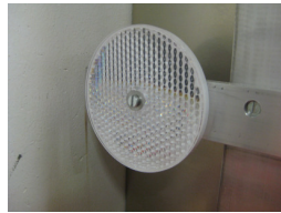
(e) The reflector mirrors the signal coming from the emitter back to the acceptor.
