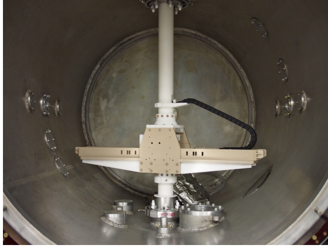
Figure 6.1: Mapping device located inside the vacuum tank.
