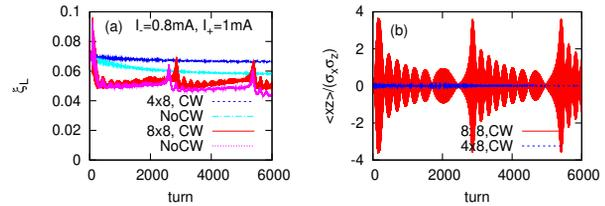
Figure 1: Strong-strong simulation results for SuperKEKB [1]. (a) and (b) show the beam-beam parameter and head-tail motion  $\langle xz \rangle$ , respectively, at the commissioning stage with IP beta,  $(8\times, 8\times)$ , and  $(4\times, 8\times)$ .
