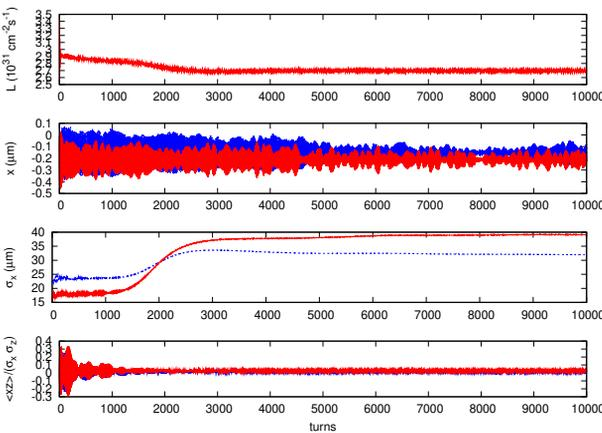
Figure 3: Evolution of luminosity, dipole moment  $\langle x \rangle$ , beam size  $\sigma_x$  and correlation of  $\langle xz \rangle$  given by the strong-strong simulation. Those of positron and electron beams are plotted with red and blue lines, respectively. Tune is  $\nu_x^{(+)} = 0.53$ ,  $\nu_z^{(+)} = 0.0247$  and  $\nu_z^{(-)} = 0.028$ .
