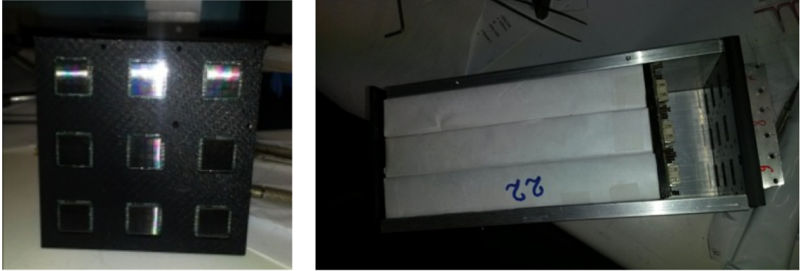
Figure 5.10: Test beam: (left) MPPC Holder, (right) matrix assembled.
