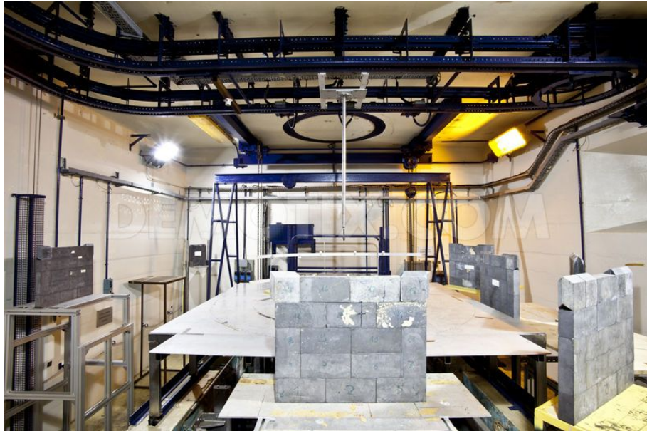
Figure 4.16: CALLIOPE gamma irradiation plant, (ENEA, Casaccia). It is a pool-type irradiation facility equipped with a ^{60}\text{Co} \gamma -source in a large volume shielded cell.
