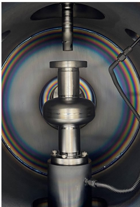
Fig. 10. 2.6 GHz Nb SRF cavity placed in the cylindrical magnetron-sputtering coating chamber for Nb-Sn multilayer deposition. The top magnetron with its target placed can be seen. The corrugated flexible line to the right is used to supply Ar gas during deposition to the discharge space.
