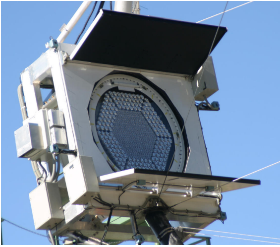
Figure 1.15: Camera of the MAGIC Telescope. Area = 0.85 \text{ m}^2 , FoV = 3.8^\circ [175].
