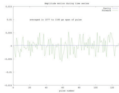
Figure 7: Preliminary results of gun amplitude feedback. The blue curve shows the stabilized field amplitude (in-loop measurement). The green curve is the input signal, and shows the work being done by the feedback system.
