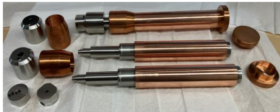
(c) Vacuum side inner conductor EB welding test
