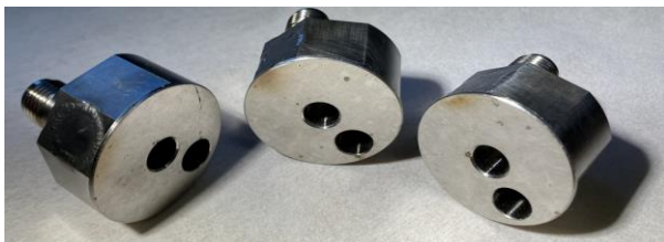
(e) Vacuum side inner conductor cooling water lead Figure 7: FPC components manufacture.
