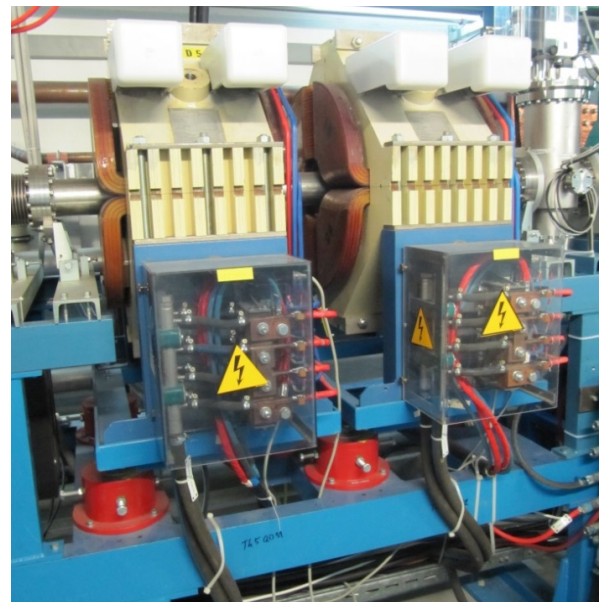
Figure 10: TK5QD5, the already existing quadrupole doublet, together with QD4 it provides a small beam spot and a double-waist on the foil to mitigate emittance growth from scattering during the stripping.
