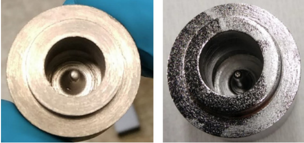
Figure 4: Machined Niobium resonators before (left) and after (right) 1:1:2 buffered chemical polishing at Argonne.
