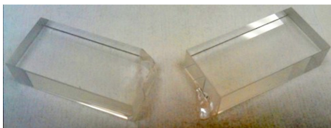
Figure 7. Broken sample with damage to the bulk sapphire.
