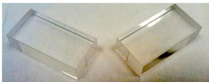
Figure 6. Sample broken across the bond.
