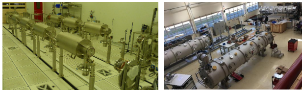
Figure 3: CM04 and CM05 cavity string in the clean room and cryomodules CM01 and CM30 (also named H-ECCTD) in the assembly hall.
