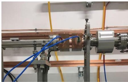
Figure 3: The installed BAM.
