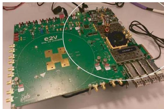
Figure 10: ADC demo board EV12AD500A.
