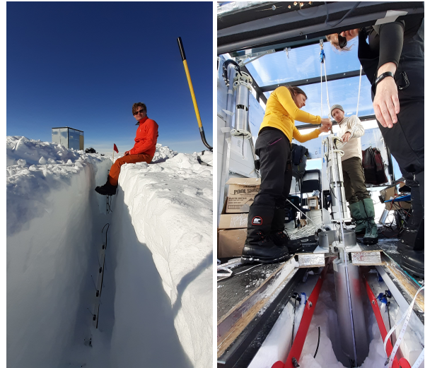
Figure 1: Layout of the hybrid RNO-G station (left) with LPDA antennas deployed in shallow trenches, and Vpol and Hpol antennas installed in the deep boreholes. The deployment process for the shallow (top-left) and deep (top-right) components, respectively, is illustrated above.
