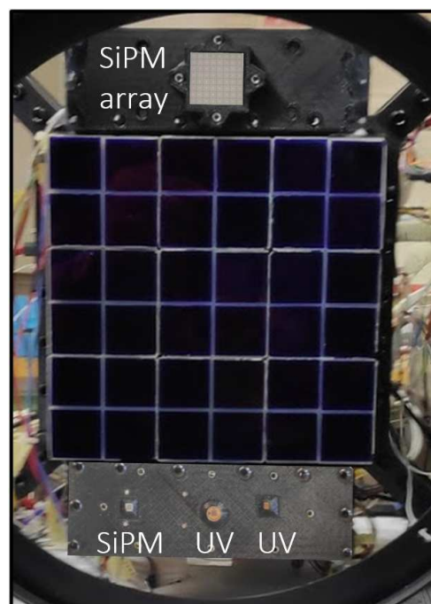
Figure 11. The Mini-EUSO focal surface. The main camera is the PDM with 36 MAPMTs. On top of the PDM there is a 64-channel SiPM array, at the bottom of the PDM there are two UV-light sensors and a single-pixel SiPM. Image adapted from Ref. [12] (© AAS. Reproduced with permission).
