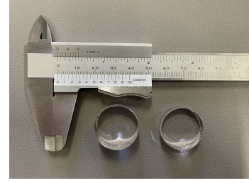
Figure 2. Quartz blanks produced for the BAUSCIA project. Left: SC-cut quartz blanks of different thicknesses (from 2 mm on the right to 27 mm on the left), used to span acoustic frequencies from a few hundred kHz to several MHz. Right: example of SC-cut quartz blanks manufactured for BAUSCIA, after the first phase of shaping and polishing.
