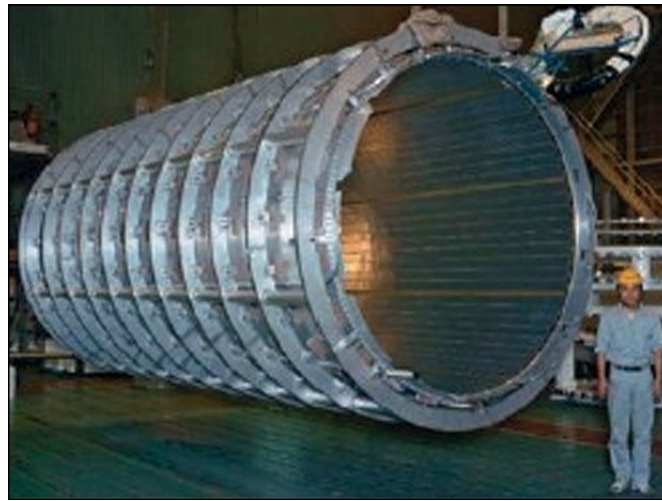
FIGURE 3.21: Bare central solenoid in the factory after completion of the coil winding.
