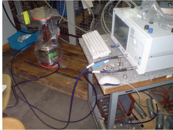
Figure 5.47: S-parameter measurement setup for the BPH.
