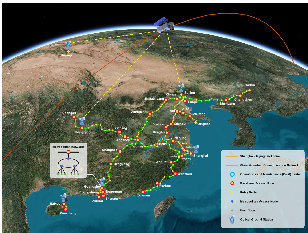
Fig. 1 | Network topology. The backbone network comprises CN-QCN (green lines) and BSNB (yellow lines). There are 145 backbone nodes, 41 (red circles) are backbone access nodes, while the remaining 104 nodes are relay nodes (yellow dots). The
