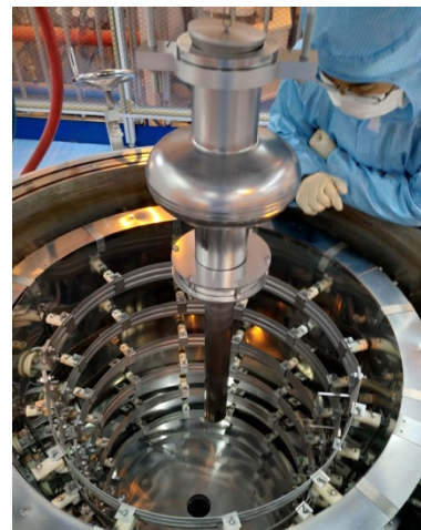
Figure 1: The Nb cavity was lowered into the furnace.
