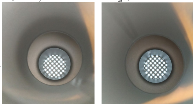
Figure 6: Typical matte grey Nb 3 Sn surface from top view (left) and bottom view (right) indicating uniform Nb 3 Sn coverage.
