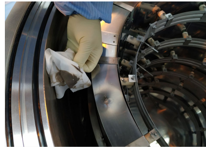
Figure 10: The inner surface of the furnace was badly polluted after each coating.
