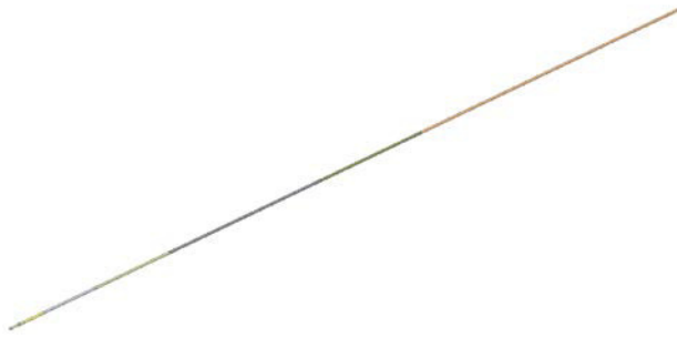
Figure 9: Segmented TFLex-405 cable model, the cold end dummy conductor locates at the left bottom corner.
