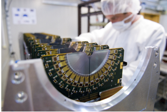
Figure 3.2 – One half of the VELO sub-detector, with its semicircular silicon modules.
