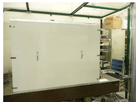
Figure 14. Newly constructed multi-layer thermal chamber.
