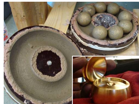
Figure 9. Demonstration of assembly and lapping and polishing of 8 brass spheres with \Delta I/I \sim 0.1
