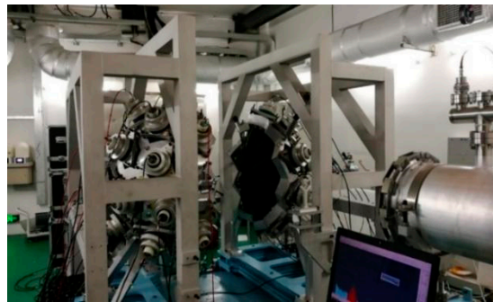
Figure 1. GTAF detector array and associated facilities installed in the Hall-2 of Back-n CSNS [6].
