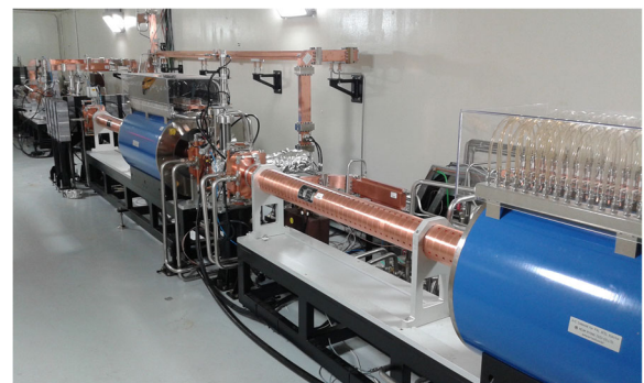
Fig. 1 Inside of the ITF tunnel. Two accelerating columns and solenoid magnets are shown
