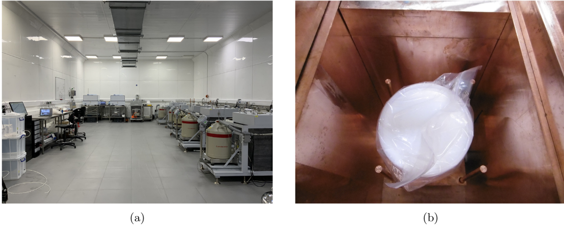
Fig. 3. (a) The BUGS Facility at Boulby Underground Laboratory and (b) a 5-kg \text{Gd}_2(\text{SO}_4)_3 \cdot 8\text{H}_2\text{O} sample on the Merrybent detector.
