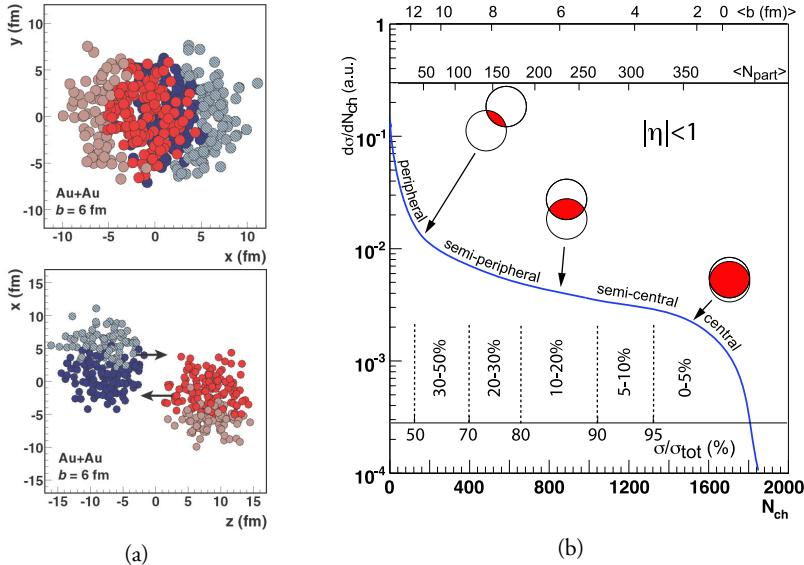
Figure 2.1: (a) Glauber Monte Carlo event of a Au+Au collision at  $\sqrt{s_{\text{NN}}} = 200 \text{ GeV}$  shown in the transverse plane (top panel) and along the beam axis  $z$  (bottom panel). The darker circles represent participating nucleons and their area corresponds to  $\sigma_{\text{NN}}$ . (b) Illustrative diagram of the dependence of final-state event multiplicity on the initial-state quantities, number of participants  $N_{\text{part}}$  and impact parameter  $b$ . [51]
