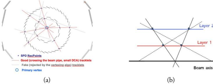
Figure 4.2: (a) Preliminary three-dimensional reconstruction of the primary vertices, also depicting tracklets rejected by the algorithm. (b) Preliminary one-dimensional reconstruction of the PVs. [141]
