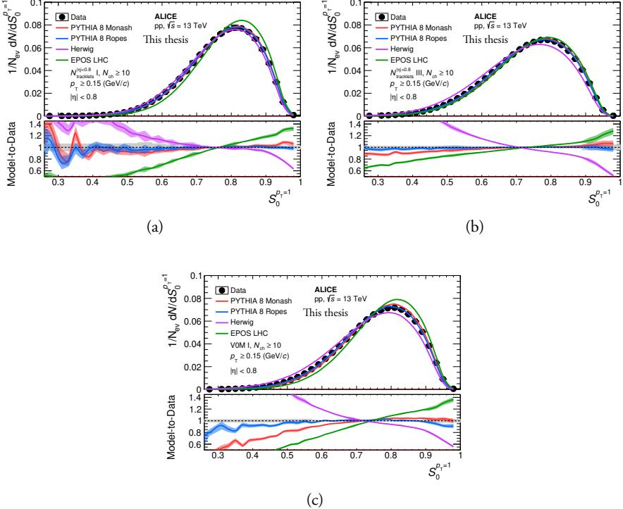
Figure 6.8: The measured and fully corrected  $S_O^{p_T=1.0}$  distributions for both (a)  $N_{\text{tracklets}}^{|\eta|<0.8} 0\text{--}1\%$ , (b)  $0\text{--}10\%$  and (c) VOM  $0\text{--}1\%$ . The curves represent different model prediction, where the shaded area represents the statistical uncertainty of the models. Plots co-produced with co-author O. Vazquez.
