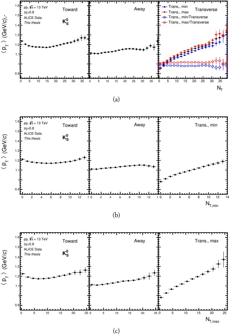
Figure 7.16: Mean transverse momentum for  $K_S^0$  as a function of (a)  $N_T$ , (b)  $N_{T,\min}$ , (c)  $N_{T,\max}$  in the different azimuthal regions. The x-axis ranges were chosen such that they represent comparable quantiles of the distributions of their variables, to facilitate a more direct comparison. Only statistical uncertainties are presented and systematic biases on  $\langle p_T \rangle$  from the unfolding treatment were not considered.
