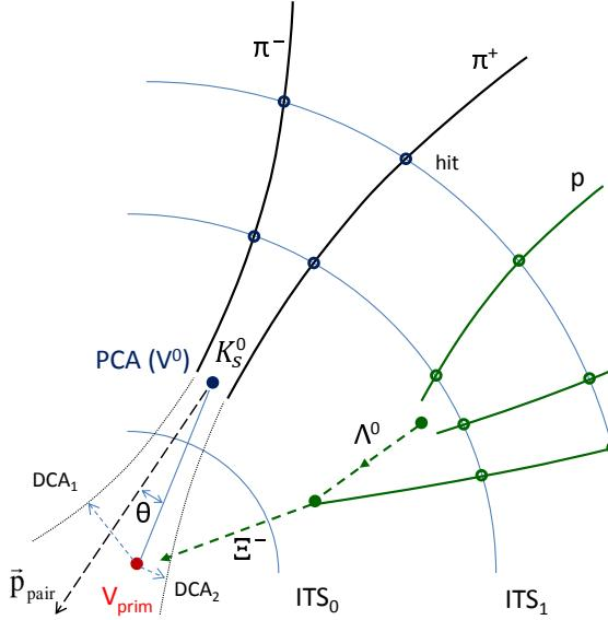
Figure 4.5: Diagram showing topology of a  $V^0$  decay (in this case  $K_S^0$ ) and a cascade decay (in this case  $\Xi$ ) in the central barrel. Here, the decays occurred within the ITS volume, but this is not a requirement for the reconstruction. The radii are not to scale. [132]
