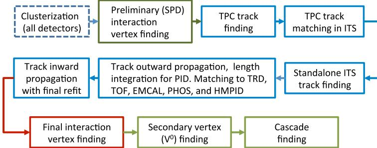
Figure 4.1: Work flow diagram of the event information reconstruction in the central barrel. [130]
