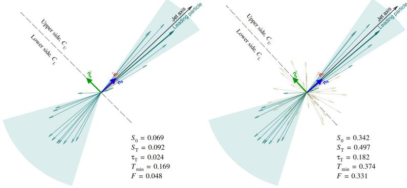
Figure 6.1: Visualisation of two events in the azimuthal plane: **(left)** more “jetty” and **(right)** more isotropic. Values for the transverse spherocity  $S_0$  are given as well as for some other event shape observables: sphericity, thrust, thrust-minor, and  $F$ -parameter. The vector minimising the  $S_0$  calculation is denoted as a blue arrow. [153]
