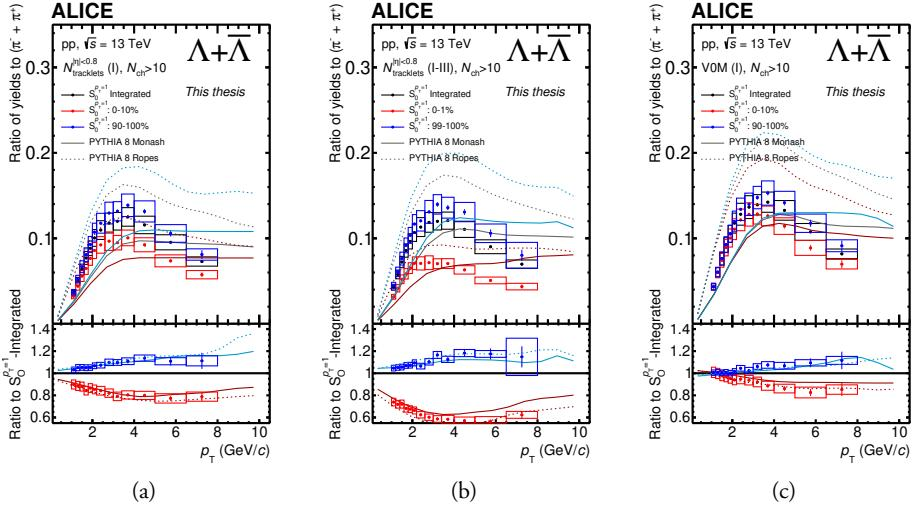
Figure 6.19: Ratios of transverse momentum spectra of  $\Lambda + \bar{\Lambda}$  to  $\pi^+ + \pi^-$  in jetty, isotropic, and  $S_O^{PT=1.0}$ -unbiased in events with high-multiplicity classes (a)  $N_{\text{tracklets}}^{|\eta|<0.8}$  I, (b)  $N_{\text{tracklets}}^{|\eta|<0.8}$  I-III, and (c) V0M I. Statistical and systematic uncertainties are depicted as error bars and boxes, respectively.
