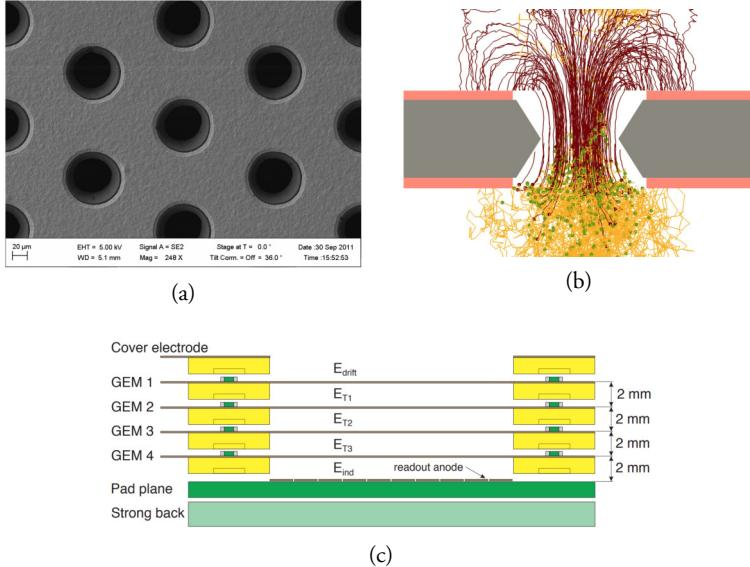
Figure 3.5: (a) Electron microscope photograph of a GEM foil with hole pitch  $140\ \mu\text{m}$ . [134] (b) Simulation of the charges in GEM holes. Dark lines represent ions and light lines electrons. Green dots mark multiplication site. (c) Schematic of the GEM setup at the upgraded ALICE TPC. [133]
