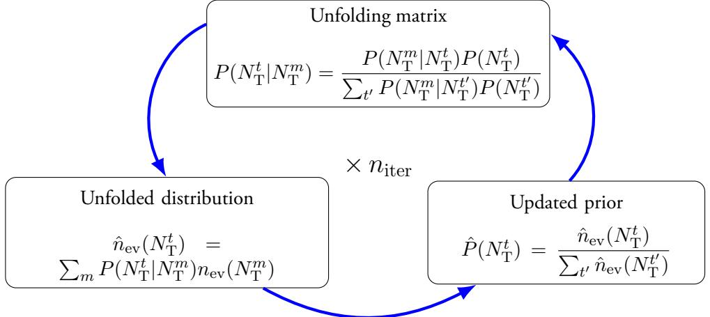
Figure 7.9: Diagram showing the iterative process of Bayesian unfolding.
