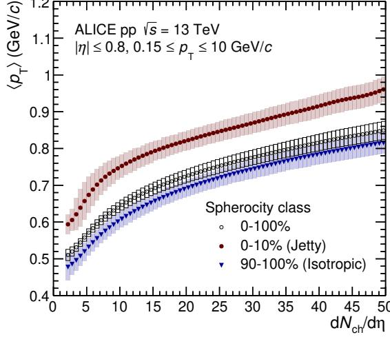
Figure 6.2: Dependence of the average transverse momentum of charged particles on the event multiplicity at mid-rapidity. Results for jetty, isotropic, and spherocity-unbiased events are displayed. Systematic uncertainties are indicated by the boxes and shaded areas. [155]
