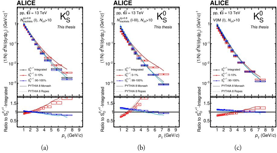
Figure 6.13: Transverse momentum spectra of  $K_S^0$  in high-multiplicity jetty (red) and isotropic (blue) events of pp collisions at  $\sqrt{s} = 13$  TeV measured in the (a)  $N_{\text{tracklets}}^{|\eta|<0.8}$  I, (b)  $N_{\text{tracklets}}^{|\eta|<0.8}$  I-III, and (c) V0M I event classes. The bottom panels display ratios to the  $S_0^{P_T=1.0}$ -unbiased spectra. Statistical and systematic uncertainties are indicated with error bars and boxes, respectively.
