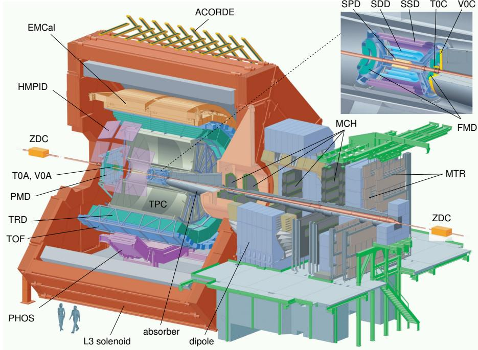
Figure 3.2: The ALICE experiment at the LHC, showing its sub-systems. The central barrel is subjected to a magnetic field from the solenoid (red). The ZDC detectors are approximately  $\pm 113$  m distant from the IP. [132]
