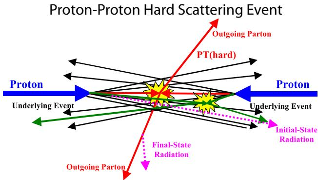
Figure 1.12: Cartoon illustrating a  $pp$  collision and its components: the hard scattering process, beam remnants, initial/final state radiation, and the MPIs. The last three contribute to the underlying event. [32, 34]
