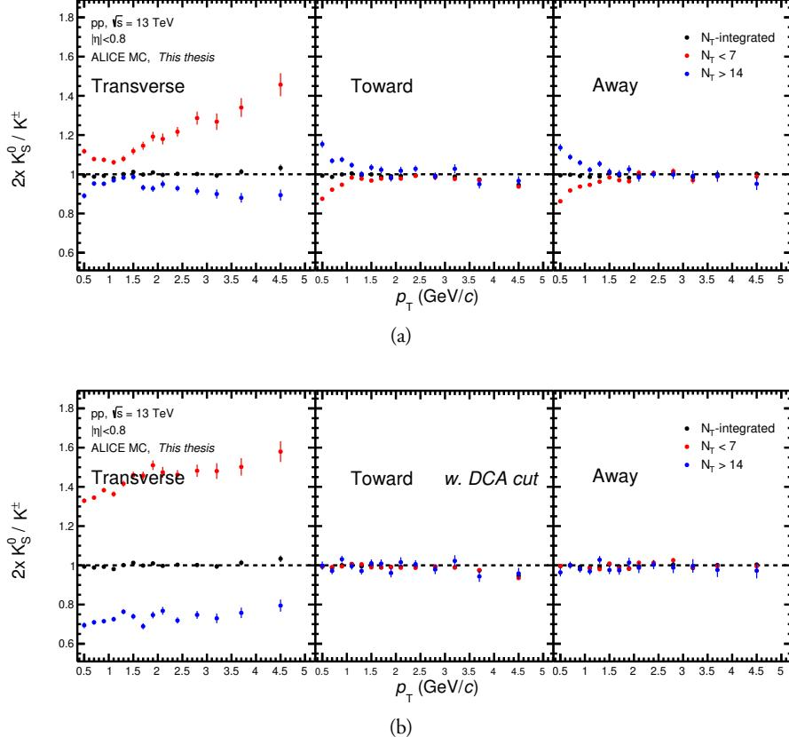
Figure 7.7: Transverse momentum spectra ratios of the neutral  $K_S^0$  to the charged  $K^\pm$  without enforcing the DCA cut (top) and after its inclusion (bottom) in the three azimuthal regions. Events with low  $N_T$  (red) and high  $N_T$  (blue) are compared. The results come from ALICE detector simulations, are uncorrected for reconstruction effects and acceptance, and show only statistical uncertainties.
