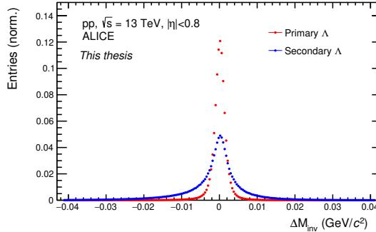
Figure 5.5: Invariant mass distributions of primary  $\Lambda$  (red) and secondary  $\Lambda$  (blue) in ALICE MC simulations of  $pp$  collisions at  $\sqrt{s} = 13$  TeV
