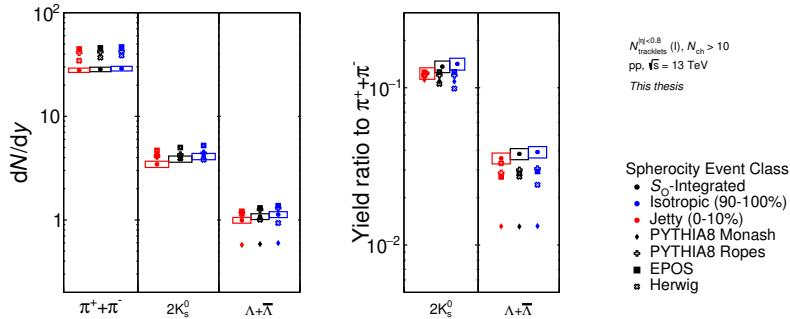
Figure 6.17: Integrated yields of  $\pi^+ + \pi^-$ ,  $K_S^0$ , and  $\Lambda + \bar{\Lambda}$  in jetty, isotropic, and  $S_O^{p_T=1.0}$ -unbiased high-multiplicity events determined at mid-rapidity, and the ratios of  $K_S^0$  and  $\Lambda + \bar{\Lambda}$  to pions.
