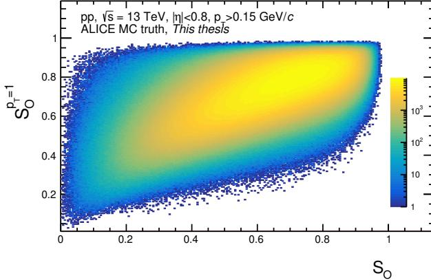
Figure 6.6: Two-dimensional histogram showing the correlation between the traditional transverse spherocity  $S_O$  and the unweighted transverse spherocity  $S_O^{p_T=1.0}$  employed in this measurement, obtained from ALICE MC simulations.
