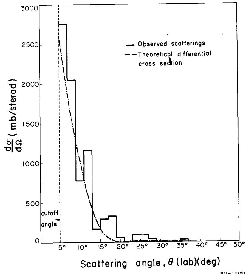
Fig. 11.  $\bar{p}$ -C differential scattering. This is a histogram showing our  $\bar{p}$ -C elastic-scattering differential cross section including all events of antiproton kinetic energy between 75 and 200 Mev. An optical-model curve due to Bjorklund and Fernbach, using the method of Watson and Riesenfeld and the Ball-Chew phase shifts for 140 Mev, is also shown.
