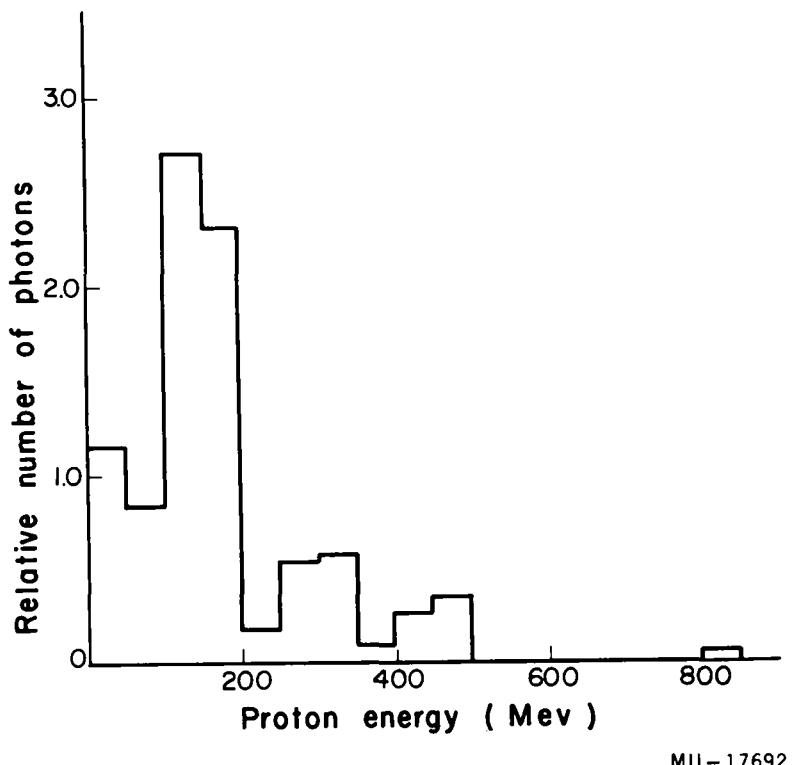
Fig. 15. Energy histogram of 29  $\pi^0$ -decay  $\gamma$  conversions observed in hydrogen annihilations. Each photon has been weighted according to its conversion probability. Because of the effect of the weighting factor, each unit of the ordinate represents 50 photons.
