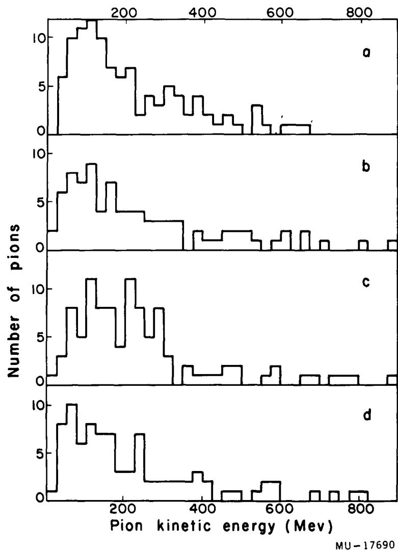
Fig. 16. Kinetic-energy spectra of charged pions from carbon annihilations. Only pions with at least 10 cm of track (unless stopping) and which make an angle of  $\gtrsim 60^\circ$  with the magnetic field are included.
