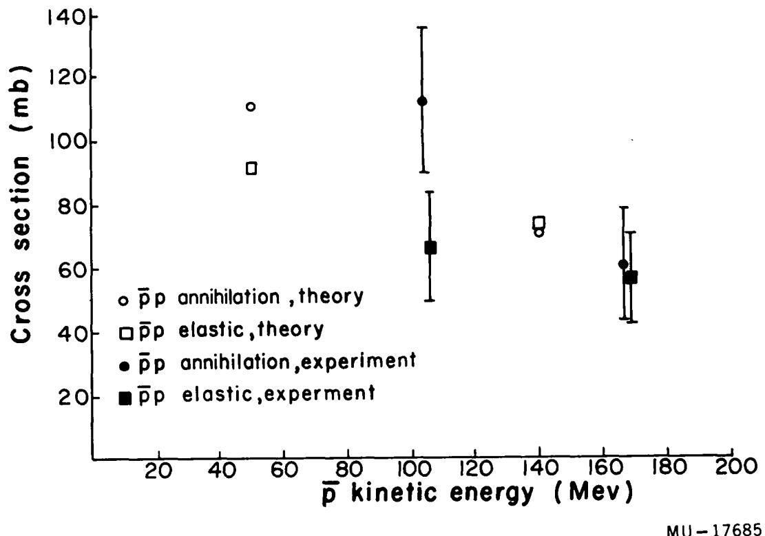
Fig. 7.  $\bar{p}p$  cross sections. A comparison of theoretical (Ball-Chew model) and experimental  $\bar{p}p$  elastic and annihilation cross sections. The experimental points are averages over two energy intervals, 75 to 137.5 Mev, and 137.5 to 200 Mev.
