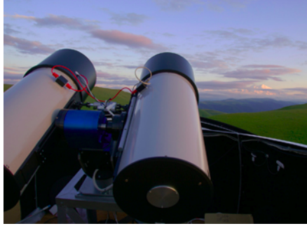
Figure 3.18: The MASTER Kislovodsk telescope in Russia, which consists of two wide FoV telescopes.
