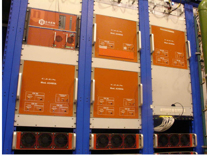
Figure 2.20: One of the four ALICE TOF rack low-voltage subsystems with the SY1527 mainframe, the A1395-Service and three A1395A-Power power supplies.
