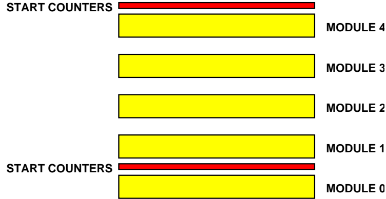
Figure 3.13: Scheme of the CRTF showing the position of TOF modules and of the START trigger scintillator layers.
