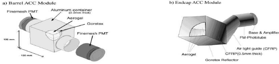
Figure 2.14: Schematic drawing of a typical ACC counter module: (left) barrel ACC (right) endcap ACC [39]
