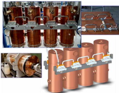
Figure 3: New cavities support system inside cryostat improved alignment and cooling performances.
