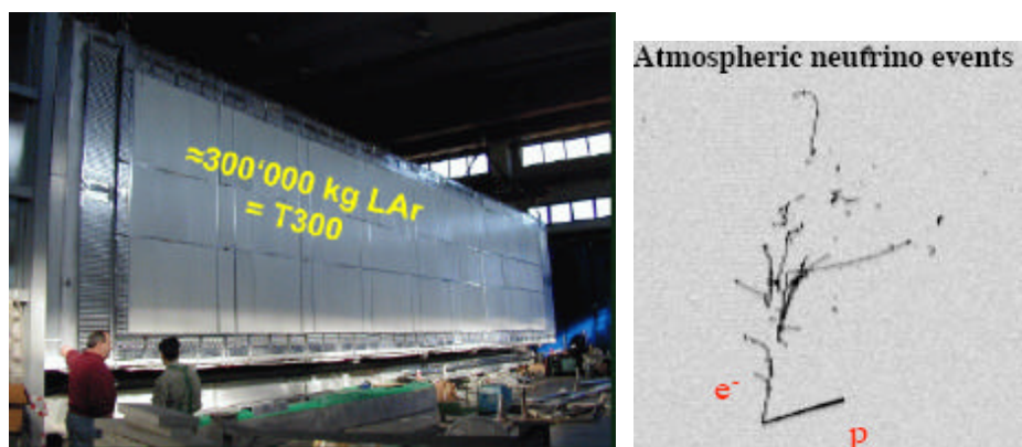
Figure 12a and 12b The ICARUS TPC in the Gran Sasso tunnel and a typical event.
