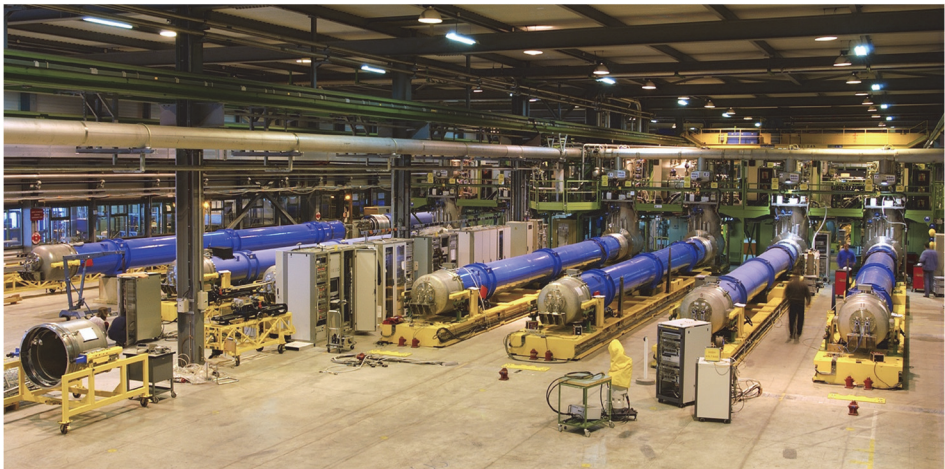
Fig. 11.7. Cryogenic test station for reception tests of LHC main magnets.
