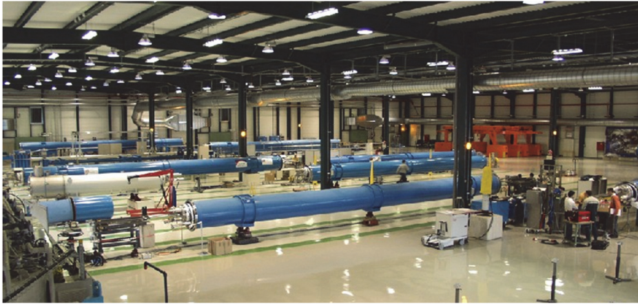
Fig. 11.8. Assembly of LHC superconducting magnets into their cryostats.
