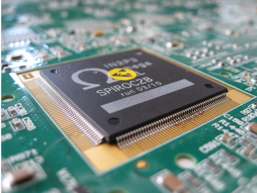
Figure 2.7: A SPIROC2b ASIC mounted on a HBU PCB.
