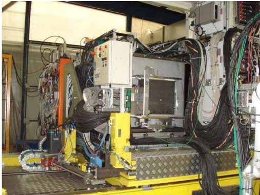
(a) CALICE detector setup consisting of ECAL (front) AHCAL (center) and TCMT (rear) in the test beam at Fermilab.
