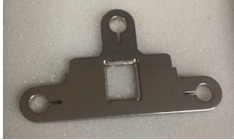
Figure 2.12: The impact plate with a hole for embedding of SSD.
