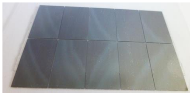
Figure 5.53: Picture from the back side of a gluing test with 3M double side tape of a dummy detector on top of a glass piece.
