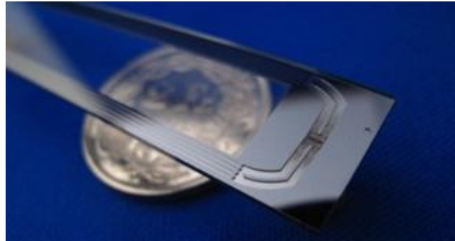
Figure 1.10: Micro-channel frame design for the ALICE ITS upgrade (Ref. [20]).
