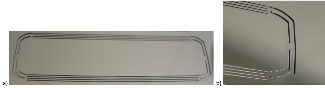
Figure 4.15: ALICE micro-channel frame design (a) with the magnification of the distribution manifold (b).
