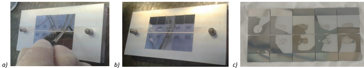
Figure 5.50: Gluing test with Araldite 2020 deposited with a pencil (a, b), and result of the gluing (c).
