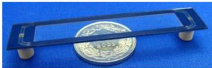
Figure 4.14: ALICE frame design with central window to reduce the material crossed by particles (Ref. [20]).
