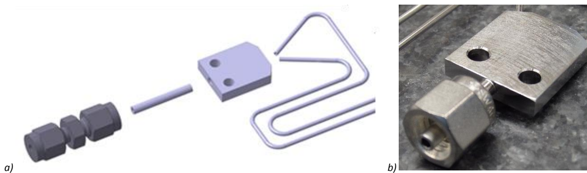
Figure 6.4: Exploded view (a) and picture (b) of the stainless steel manifold with Swagelok connector, 1/8" tube, and capillaries.
