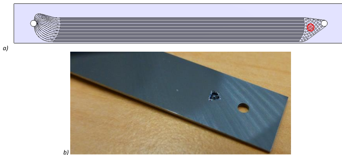
Figure 3.24: Channel design with broken area in red (a) and tested sample picture (b) of the CSEM samples done for the NA62 experiment.
