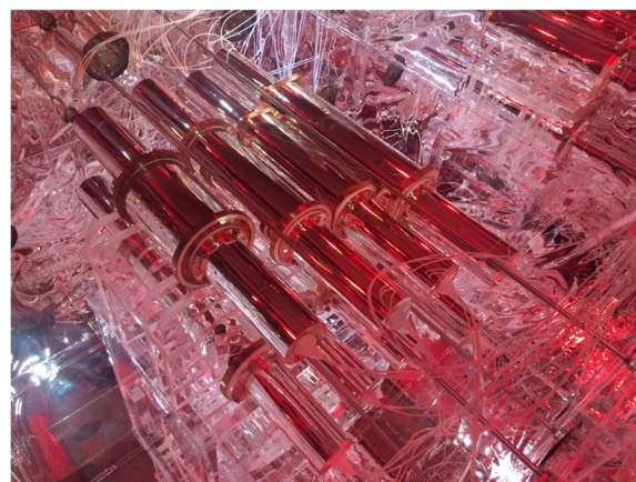
Fig. 8 Photo of NaI(Tl) crystals used for the COSINE-100 experiment
