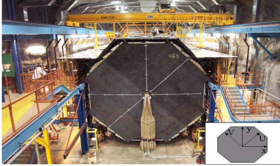
Figure 4.7: The completed MINOS far detector.
