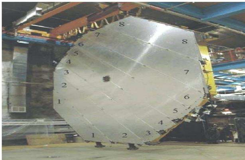
Figure 4.2: An instrumented plane of the far detector. The scintillator is encased in aluminum and is mounted on top of the steel.
