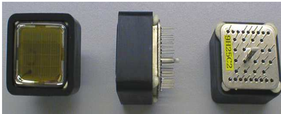
Figure 4.6: Several views of the M16 phototube.
