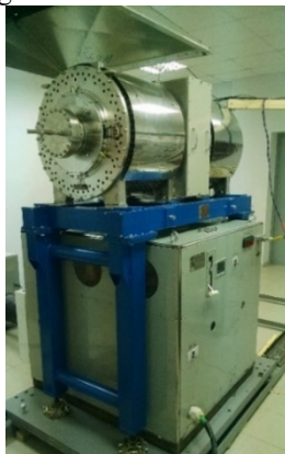
Figure 3: Booster RF station at the test bench in Dubna.
