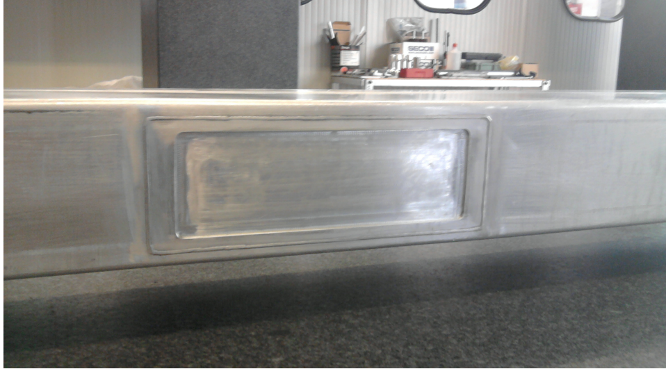
Figure 5.6: Close-up photo of the large middle window that exploded, after repair. On the upper left one can also see a repaired corner in the 3 mm aluminium sheet.
