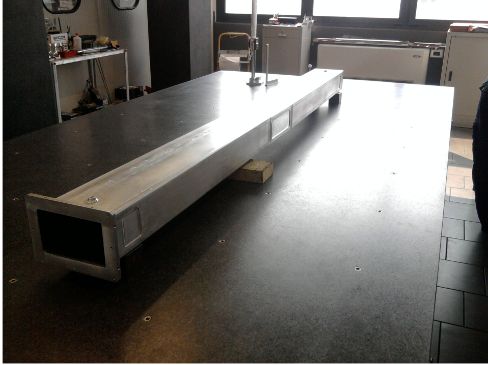
Figure 5.5: Photo of the outer shell showing the window positions on proto 2. The window sizes are chosen to admit all angles of tracks that cross the 8 layers of cells, i.e., \pm 20\text{--}30^\circ .
