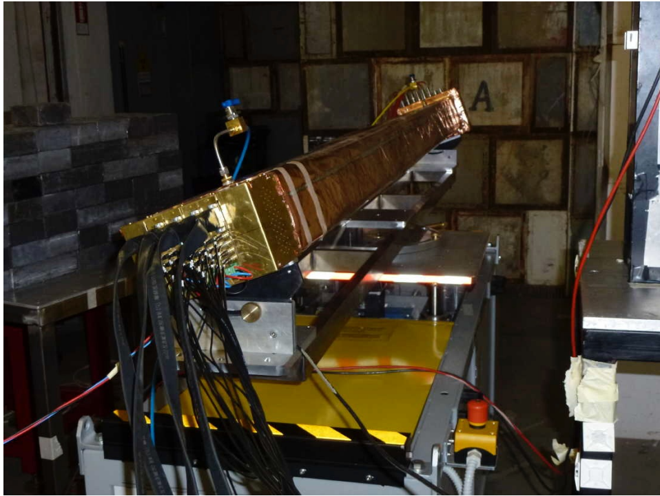
Figure 5.9: Proto 2 mounted on a movable table and tilting support, for an early beam test at LNF.
