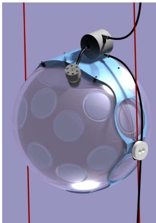
Figure 3: schematic of a DOM integrated in the detection unit
