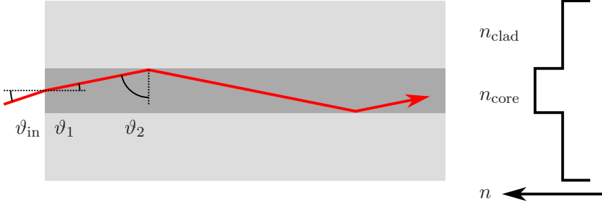
Figure 4.1: Sketch of total internal reflection (left) and the refractive index profile of a fiber (right): A beam incident at \vartheta_{in} to the fiber face will be reflected under \vartheta_2 within the fiber core. If \vartheta_2 \geq \vartheta_c is satisfied, total internal reflection occurs, and the beam is transmitted through the fiber. Otherwise, fractions of the light are diffracted into the cladding and subsequently lost. A possible refractive index profile is the step-index profile where n_{core} > n_{clad} is required to allow the total internal reflection.
