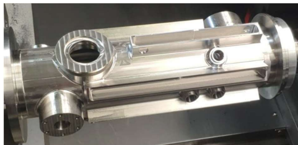
Figure 2: QWR machined from a solid billet.
