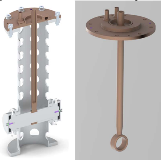
Figure 8: Stem and lid brazing with jig.
