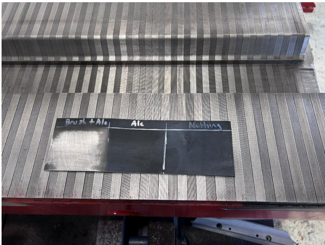
Figure 16: Lower half of a laminated H-shaped dipole on which measurements were taken and on top there is the SPS-steel sample which was prepared in three ways, going from left to right: brushed+ cleaned with alcohol, just cleaned with alcohol and no special preparation.
